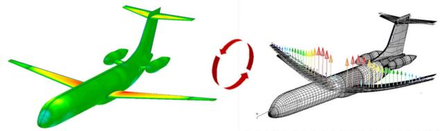
Figure 5. Fluid-Structure Multiphysics interaction of an aircraft in scFLOW and MSC Nastran
