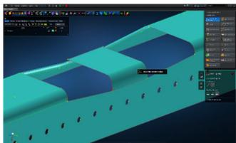
c. Defects are fixed and geometry is refined automatically
