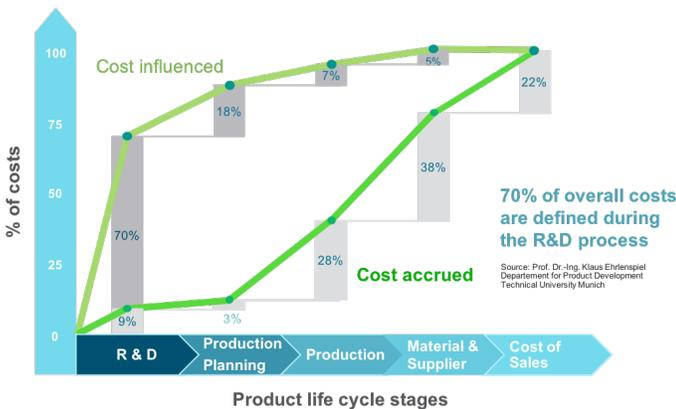
Figure 4. The relationship between costs incurred in product manufacturing versus stages of design from conception to production and deployment
