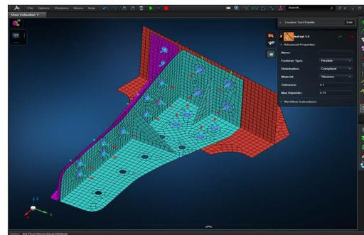
Figure 16. Leverage the simulation API to automate rivets creation on aerostructures
