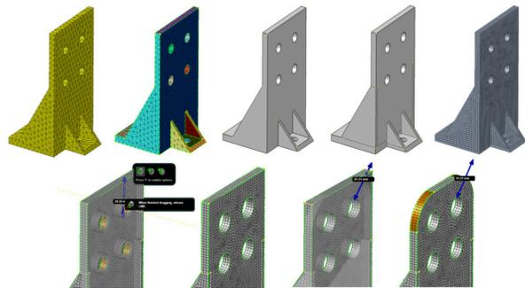
Figure 12. Regenerate geometry and recreate a Hexhedral mesh from a Tetrahedral meshed model (Top). Direct modeling on newly generated mesh (Bottom).
