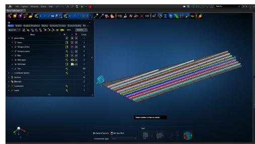
Figure 17. Automate conceptual modeling of wing structures by using MSC Apex API
